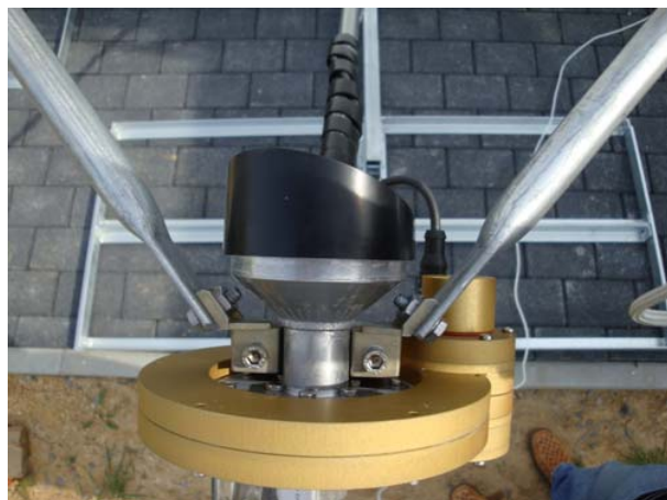
Figure 6-13: Mounted polarization drive assembly
