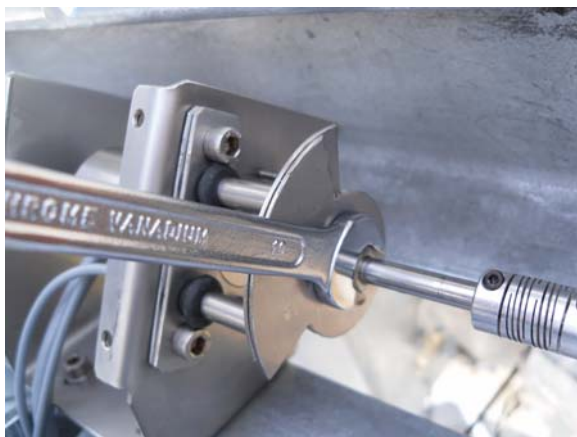
Figure 8-6/7: Elevation limit switches adjustment
